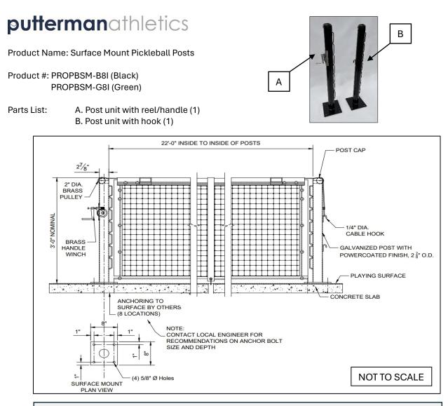
NOTE: Refer to Drawing above for layout details and post placement. Our surface mount posts are designed to be used on concrete slabs where traditional in-ground sleeves do not exist. Do not install into asphalt bases. All base slabs should be structurally sound and stable. If questions exist on the stability of the base slab, a local structural engineer should be consulted.
